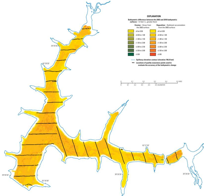
Figure 3. Bathymetric change between the 2003 survey and the 2018 survey of Sugar Creek Lake near Moberly, Missouri.
