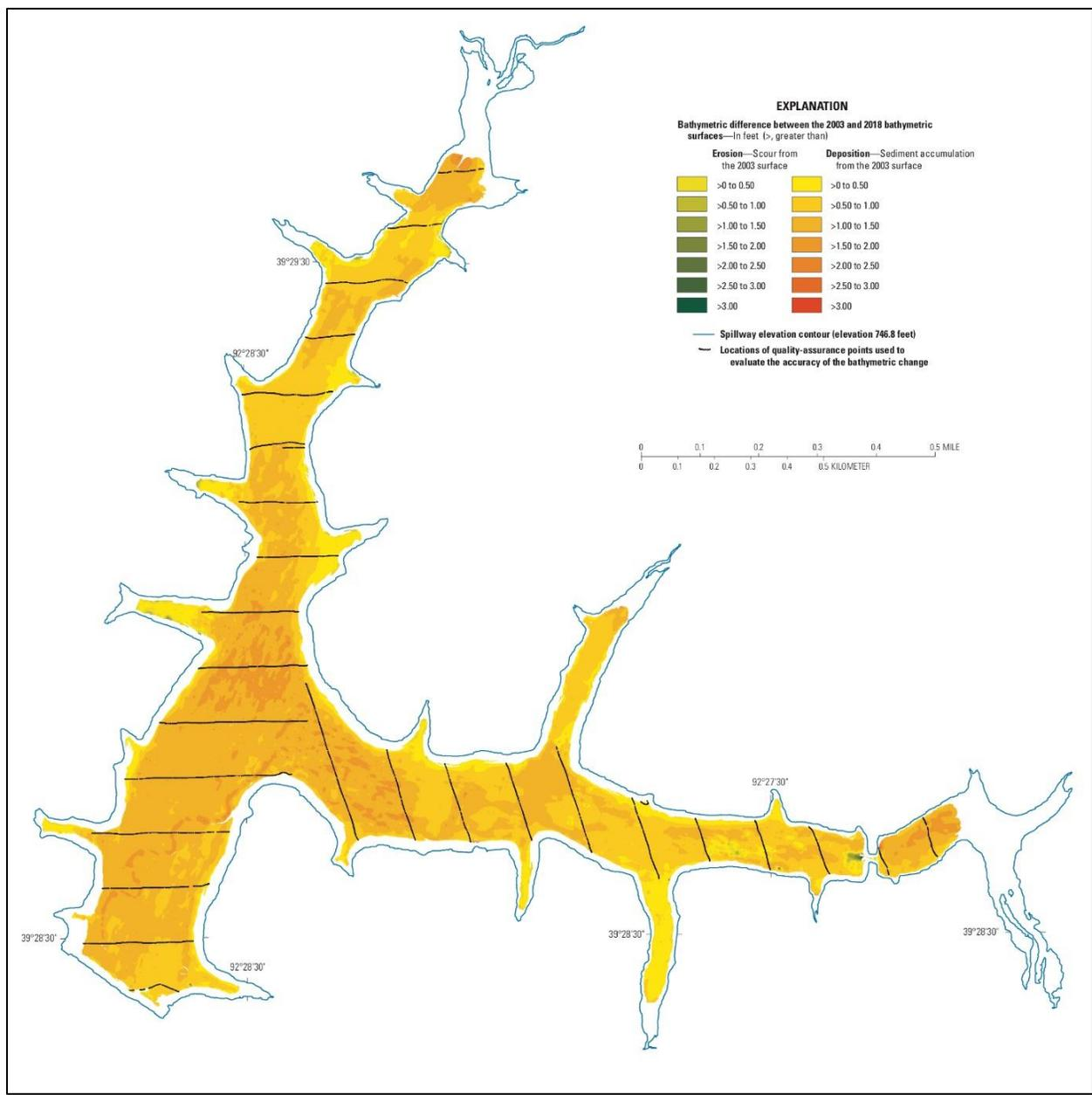
Figure 9. Bathymetric survey change since 2003 study. Change can represent either sediment deposition or erosion. Source: USGS
