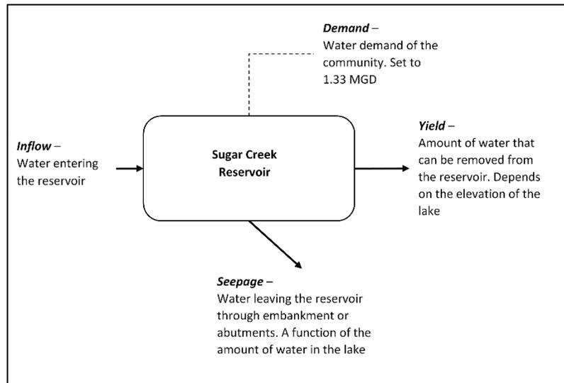
Figure 4. Schematic of water balance for Sugar Creek Lake.
