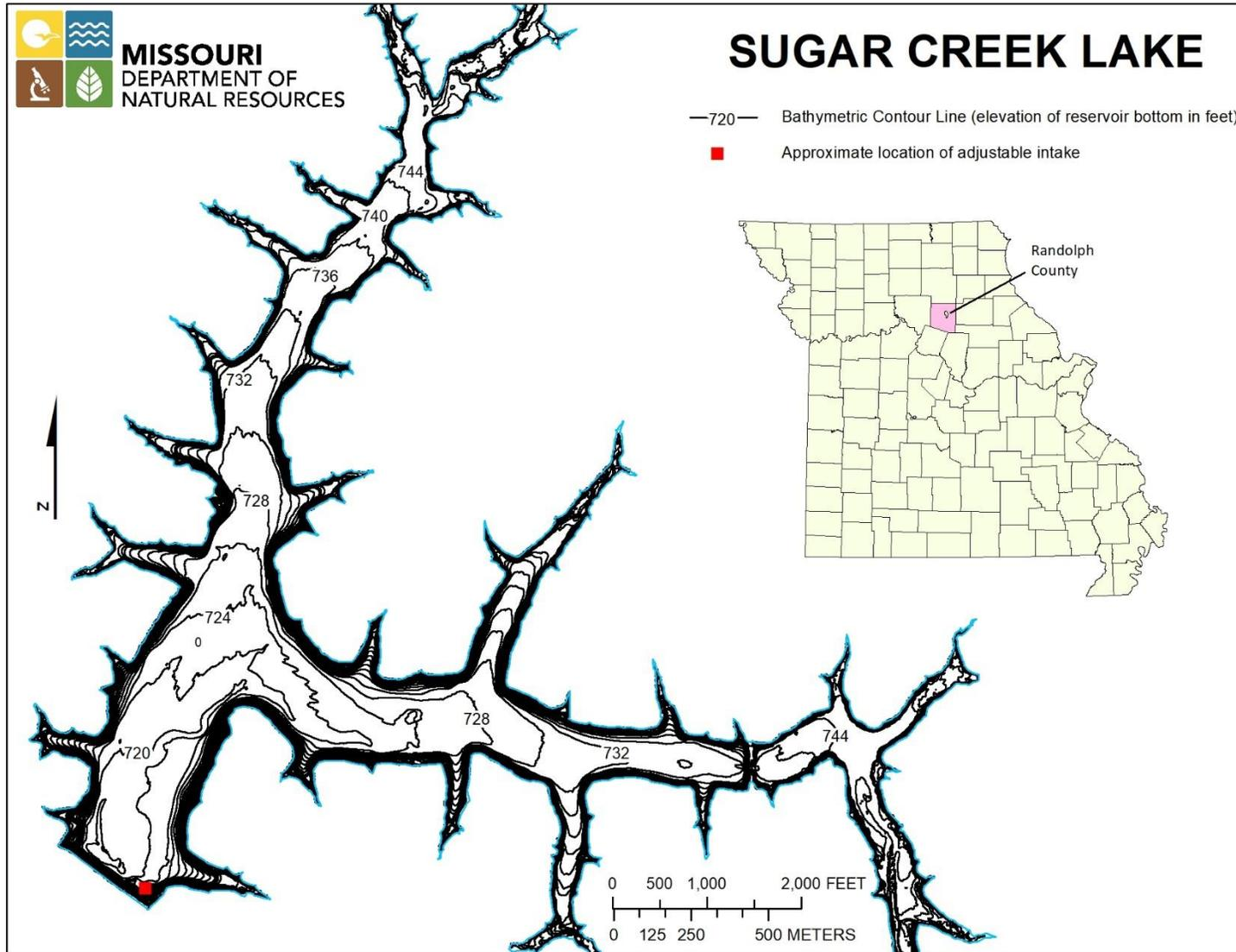
Figure 2. Bathymetric Map of Sugar Creek Lake. Contours indicate the elevation of the bottom of the reservoir as surveyed by the USGS in September of 2018. Contours are at 2-foot intervals.
