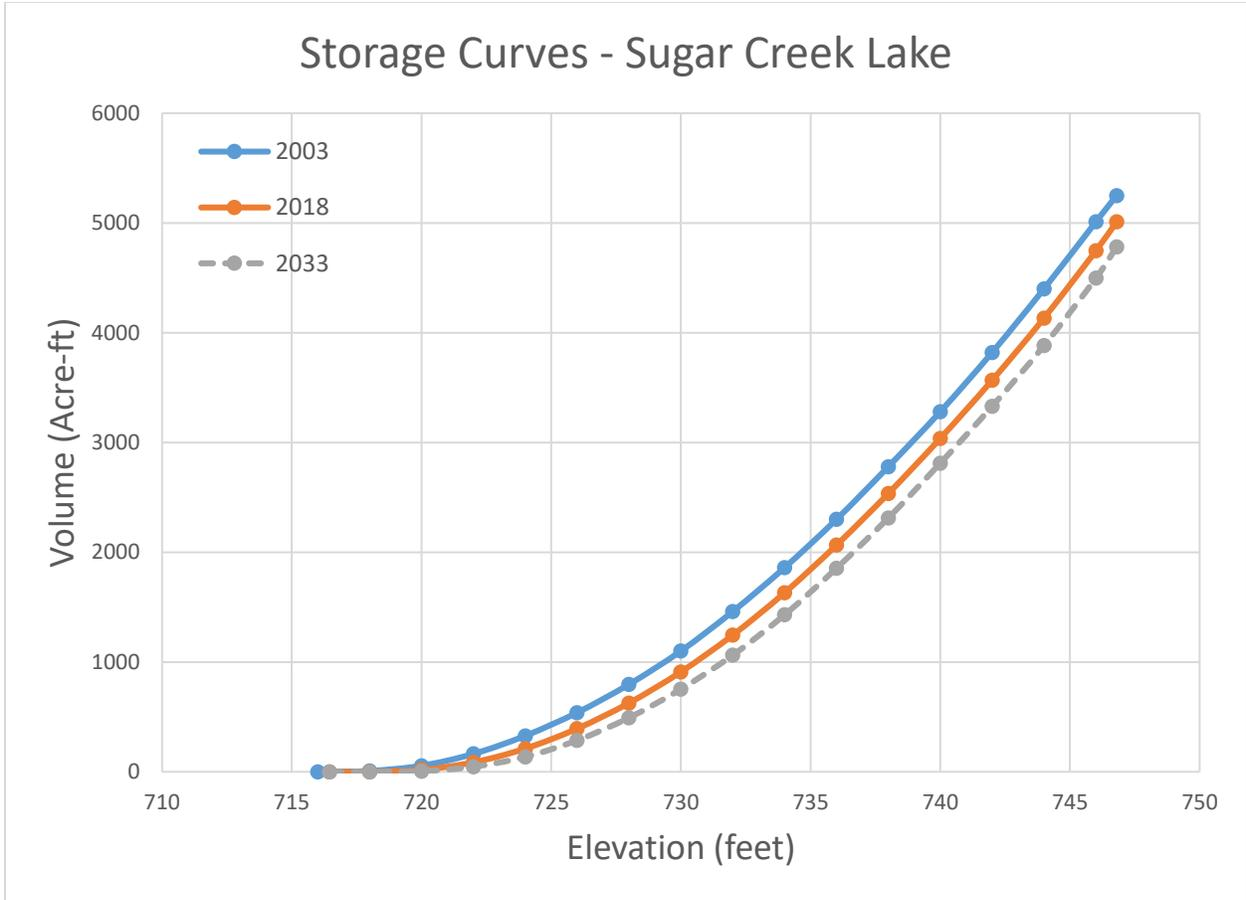
Figure 10. Storage-Elevation curves calculated from bathymetric surveys for the years 2003 and 2018. 2033 is a projected storage curve developed assuming a 4.6% loss of storage would occur from 2018 to 2033. Storage volume was lost at all elevations of the lake between surveys.
