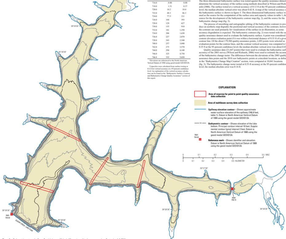
Figure 2. Bathymetric contours for Sugar Creek Lake near Moberly, Missouri, resulting from a survey done September 4-6, 2018.
