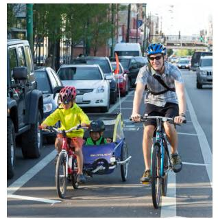
vertical separation (e.g. flex posts, parked cars, or curbs) to protect cyclist from motor traffic. The combination of horizontal and vertical separation elements can relieve most high levels of bicycle stress. The robustness of bikeway separation often scales relative to adjacent traffic volumes and speeds.
