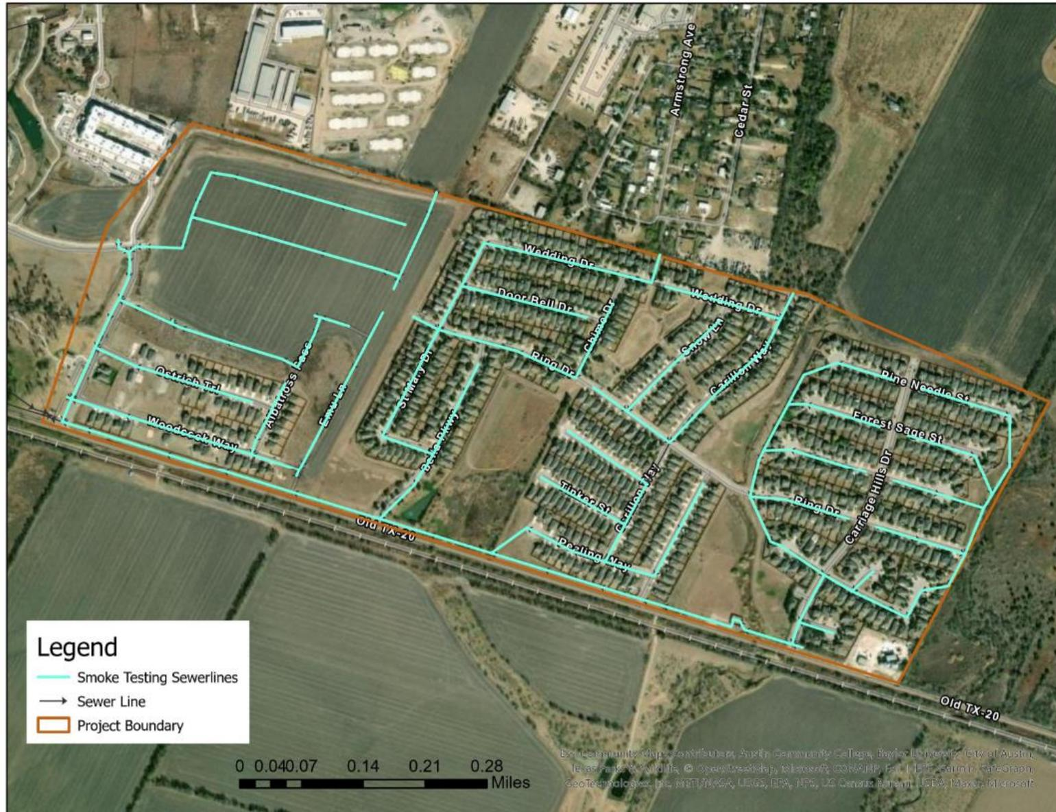
Figure 5-3 – Smoke Testing Results
