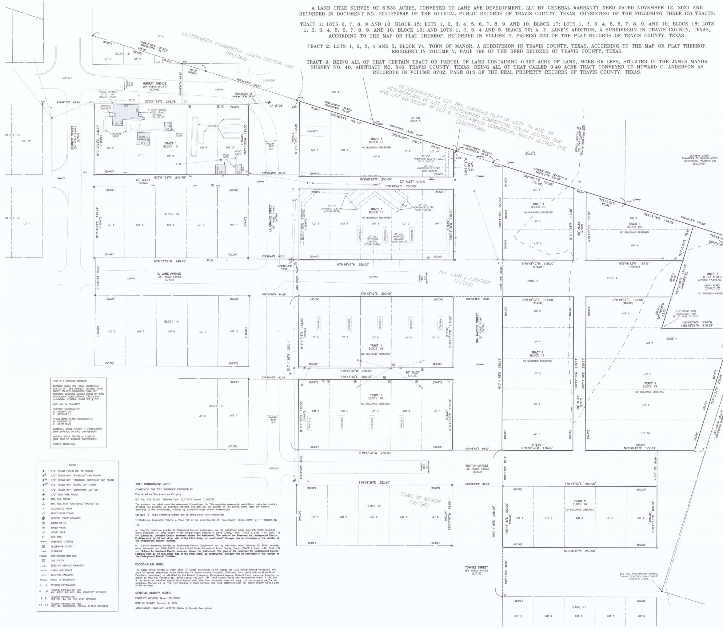
THIS IS A SURFACE DRAWING. BEARING BASIS: THE TEXAS COORDINATE SYSTEM OF 1983 (NAD83), CENTRAL ZONE, BASED ON GPS SOLUTIONS FROM THE NATIONAL GEODETIC SURVEY (NGS) ON-LINE POSITIONING USER SERVICE (OPUS) FOR CHAPARRAL CONTROL POINT "CP #103". SURFACE COORDINATES: N 1010297.23 E 3173459.11 TEXAS STATE PLANE COORDINATES: N 1010297.23 E 317341.79 COMBINED SCALE FACTOR = 0.99990010 (FOR SURFACE TO GRID CONVERSION) INVERSE SCALE FACTOR = 1.000100 (FOR GRID TO SURFACE CONVERSION) SCALED ABOUT 0.0
