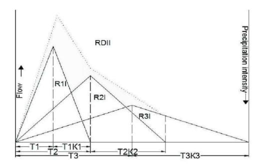
Figure 4-4: RTK Hydrograph
