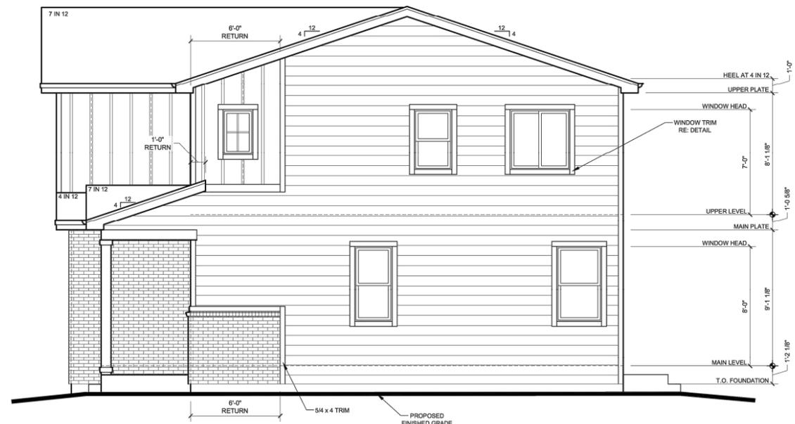
2 NON-GARAGE SIDE ELEVATION - 'A' SCALE: 1/4" = 1'-0"
