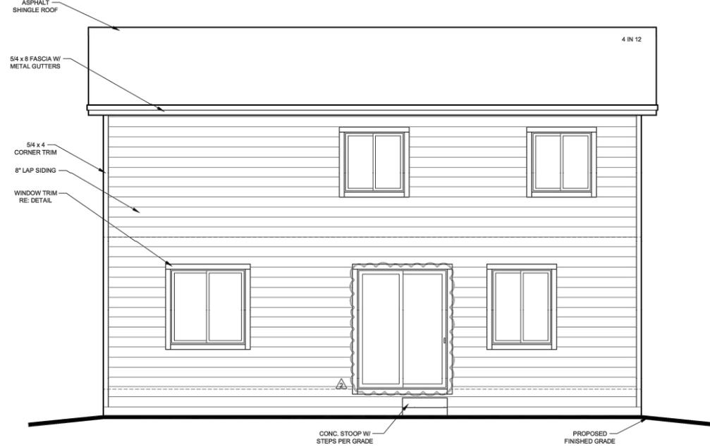
3 REAR ELEVATION - 'A' SCALE: 1/4" = 1'-0"
