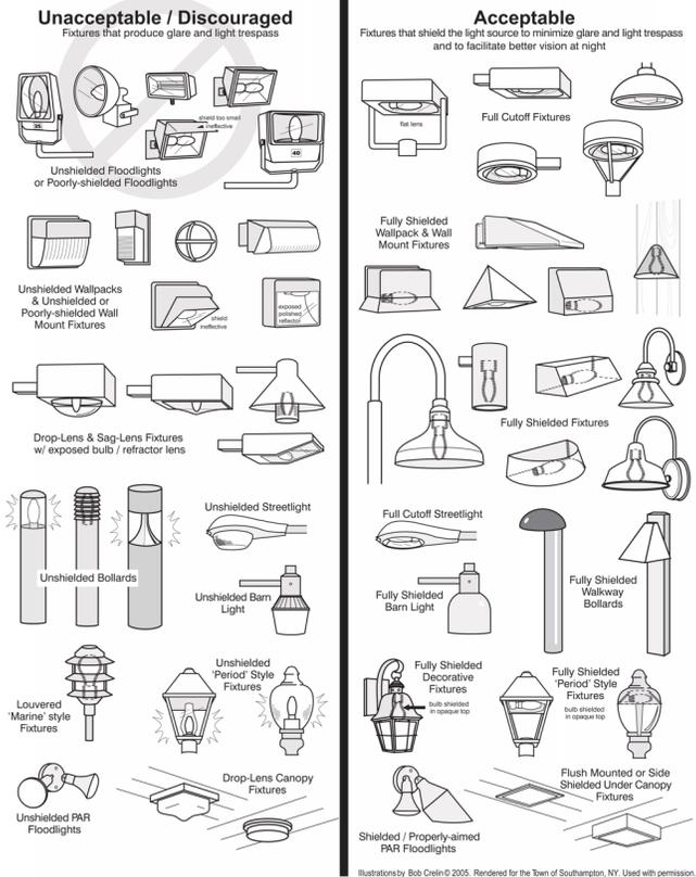
*The lights on the left are non-conforming. Those on the right can be used in most cases. Depending on the mounting height and proximity to the property line, additional shielding may be necessary to prevent the luminous elements from being visible from any other property.*
