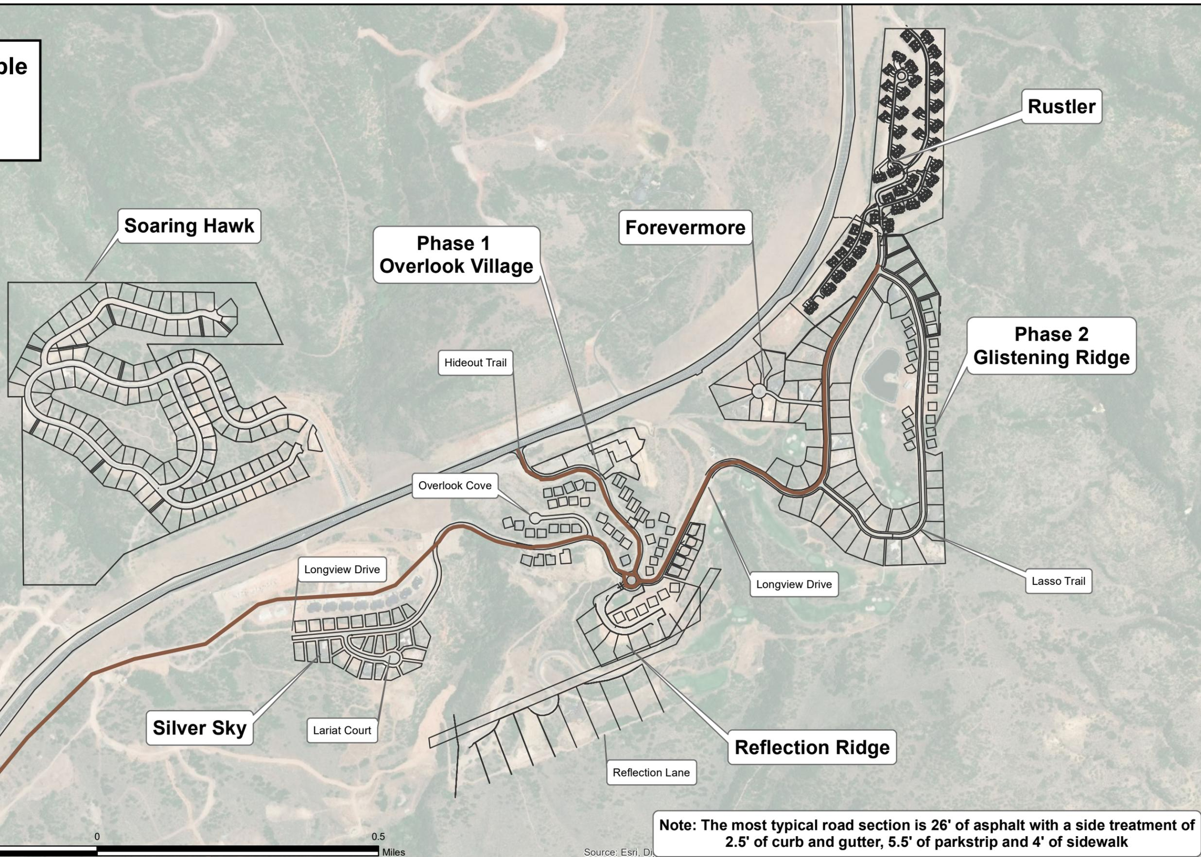
**Note: The most typical road section is 26' of asphalt with a side treatment of 2.5' of curb and gutter, 5.5' of parkstrip and 4' of sidewalk**
