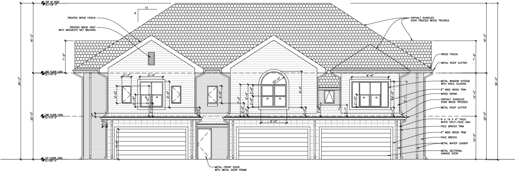
1 A2.01 TRIPLEX: FRONT ELEVATION - 80% MASONRY; 20% WOOD SIDING SCALE: 1/4" = 1'-0"
