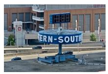
Revolving Sign. A sign which in its entirety or in part moves in a revolving manner. A SIGN that revolves three hundred sixty degrees (360°) but does not exceed eight (8) revolutions per minute.
