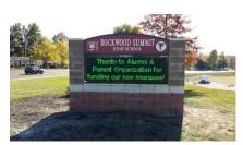
**Electronic Message Center.** A sign that is capable of displaying words, symbols, figures, or images that can be electronically changed by remote or automatic means. May also be known as a variable message sign or a LED sign.
