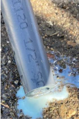
*Figure 1. Tin and chromium residuals accumulated in pipe following pilot testing of stannous chloride without filtration in Dixon, CA (2023).*
