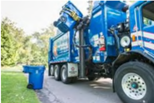
Figure 41. Preventing litter before it happens. Automated side-load trucks are designed to eliminate spillage.
