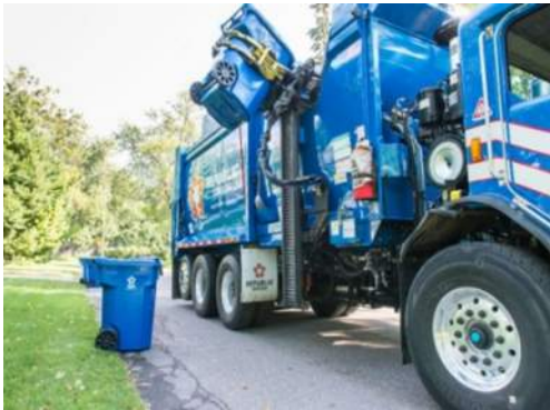
Figure 25. Automated Side Load Collection. Provides a cleaner, safer, more efficient residential collection.
