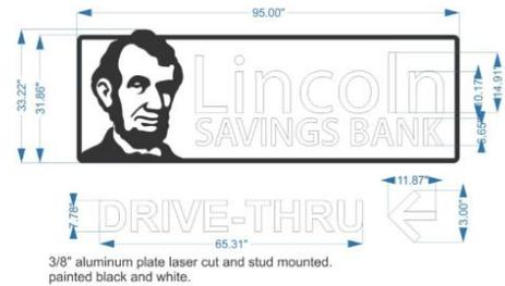
The proposed projecting sign projects about 3 feet over public sidewalk and has approximately a 12 feet clearance above the sidewalk. The sidewalk at this location is approximately 16 feet wide. The proposed placement of the sign meets city code.
