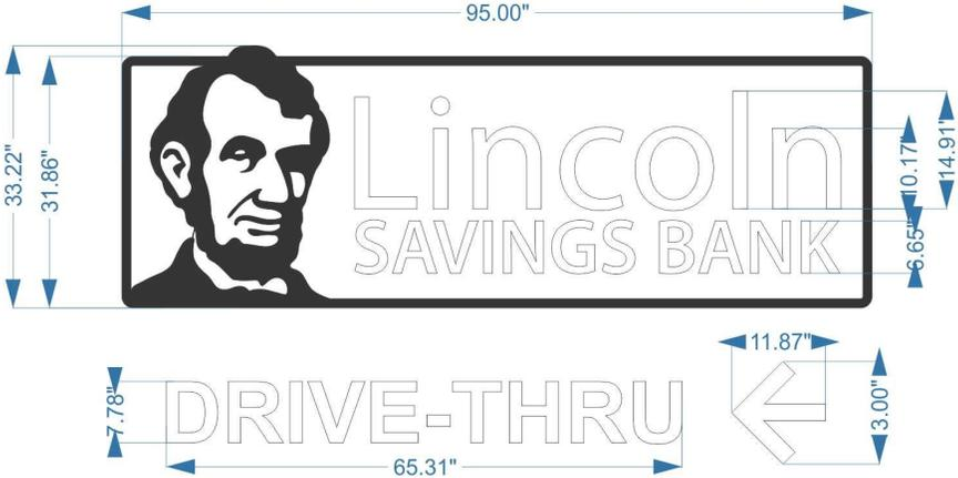
3/8" aluminum plate laser cut and stud mounted.
