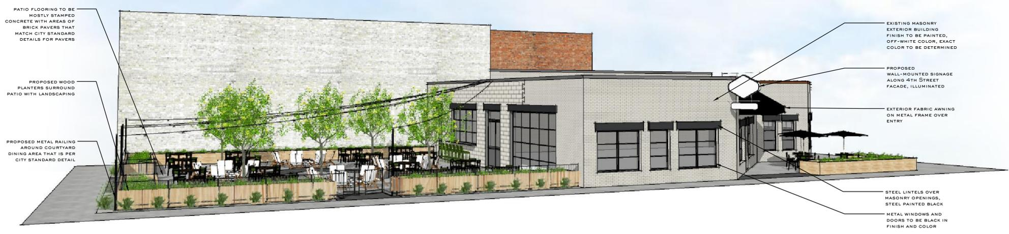
PATIO FLOORING TO BE MOSTLY STAMPED CONCRETE WITH AREAS OF BRICK PAVERS THAT MATCH CITY STANDARD DETAILS FOR PAVERS
