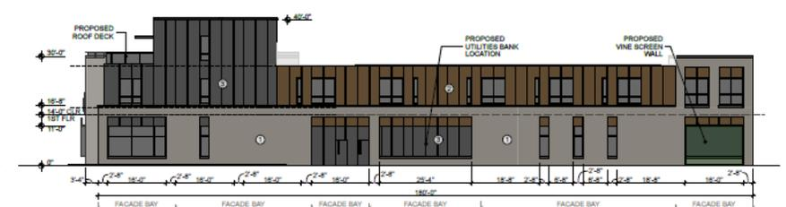
(4) NORTH ELEV. BRICK MASONRY - 49% WOOD PANEL - 29% METAL PANEL - 22% SCALE: 1" = 20'
