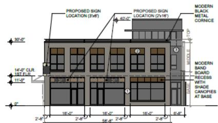
(1) EAST ELEV. BRICK MASONRY - 88% WOOD PANEL - 20% METAL PANEL - 14% SCALE: 1" = 20' STOREFRONT AS SHOWN (BW 2 & 10) - 81%
