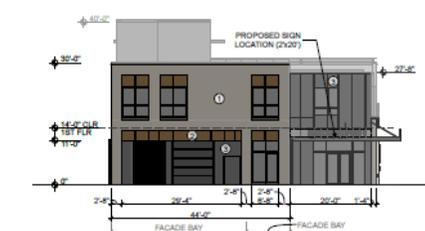
(3) WEST ELEV. BRICK MASONRY - 54% WOOD PANEL - 11% METAL PANEL - 35% SCALE: 1" = 20'
