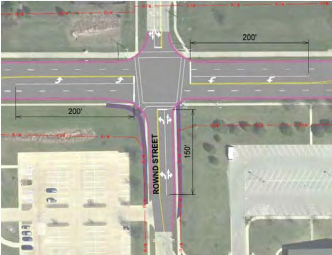
**Figure 12. Rownd St Signalized Lane Configuration**
