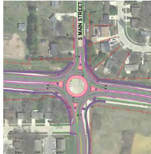
**Figure 7. S Main St Roundabout Lane Configuration**
