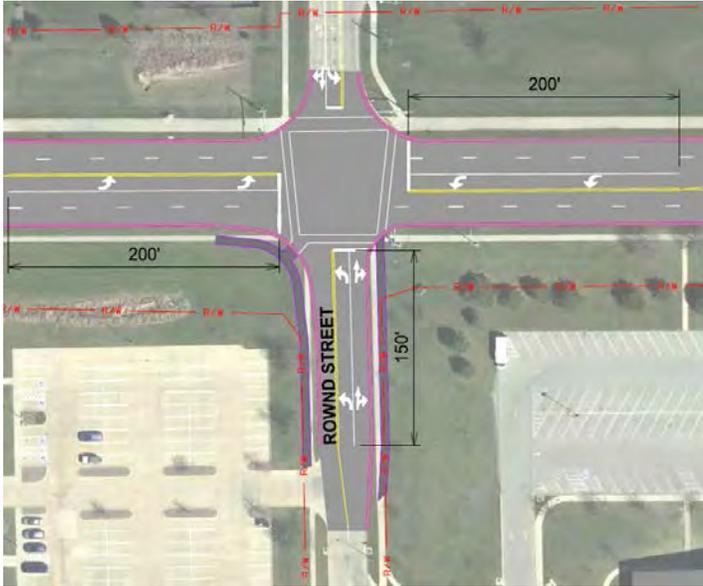
**Figure 21. Rownd St Signalized Lane Configuration**
