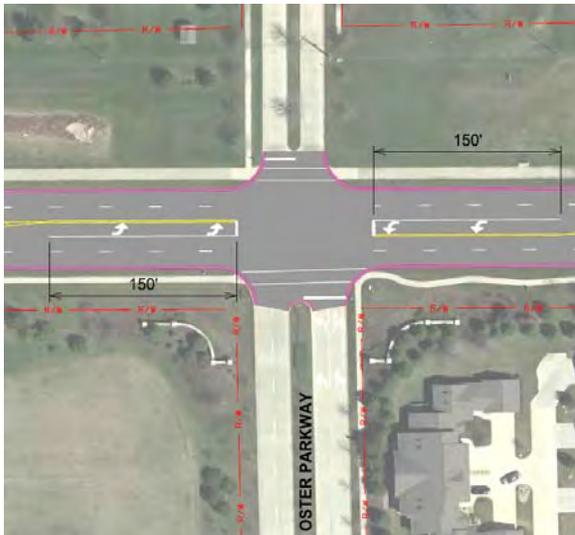
**Figure 10. Oster Pkwy Signalized Lane Configuration**
