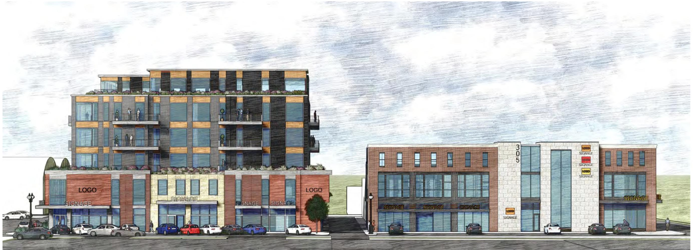
DARK TERRACOTTA PANELS    METAL PANELS    LIGHT TERRACOTTA PANELS    GRAY TERRACOTTA PANELS    LIMESTONE CLADDING    BRICK CLADDING
