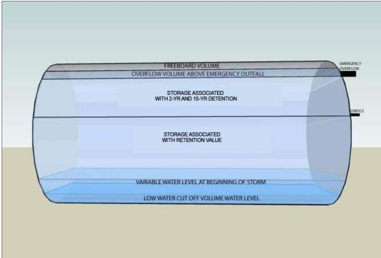
Figure 4.30. Incremental design volumes associated with cistern sizing.
