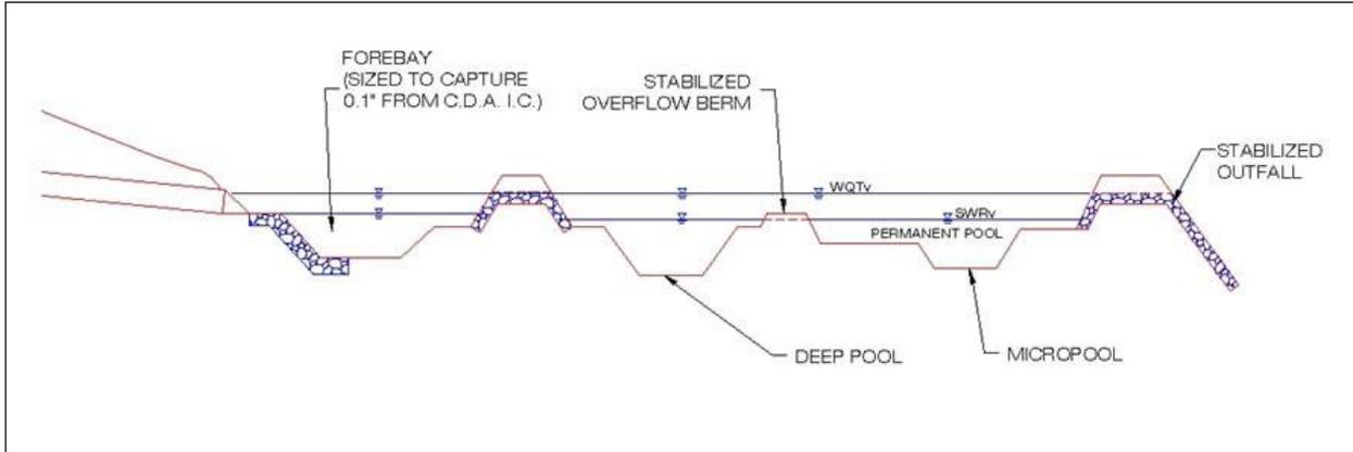
**Figure 4.54** Cross section of a typical stormwater wetland.
