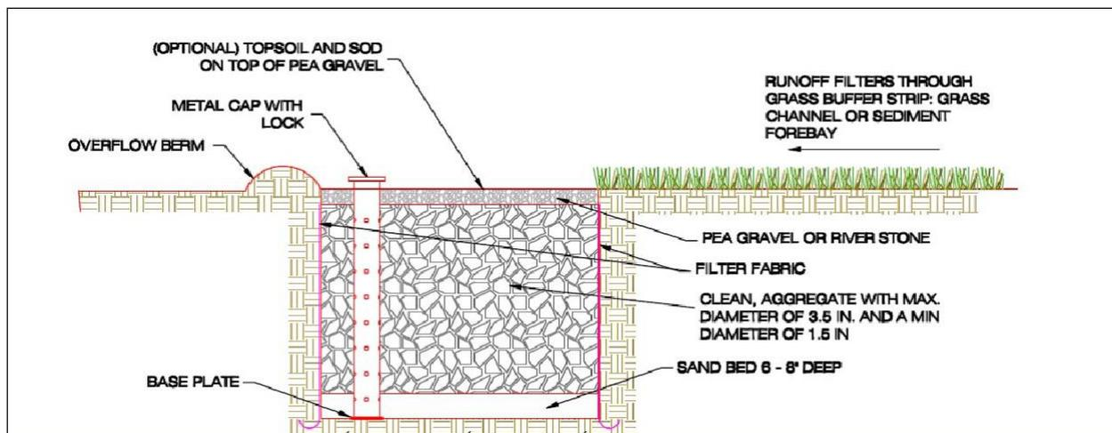
Figure 4.17. Example design of an infiltration trench.
