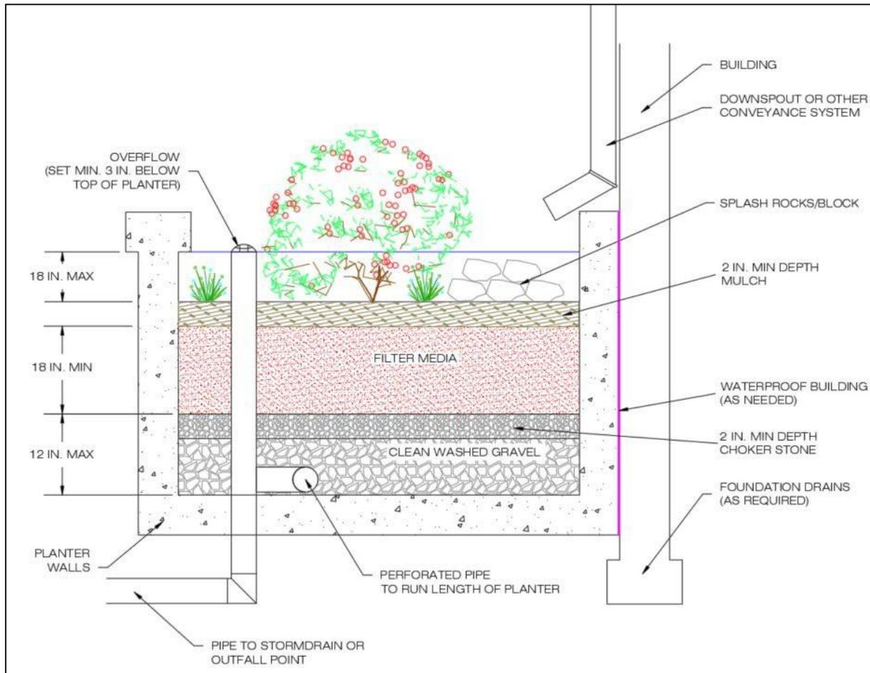
Figure 4.10. Example design of a stormwater planter (B-4).
