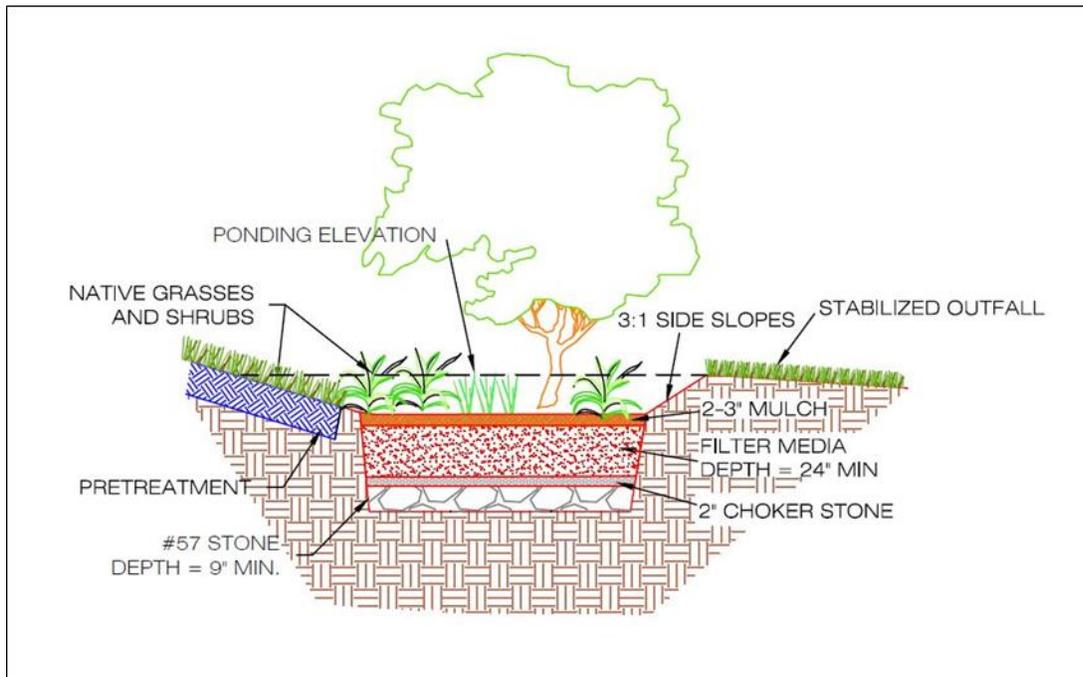
Figure 4.2. Example bioretention design without an underdrain.
