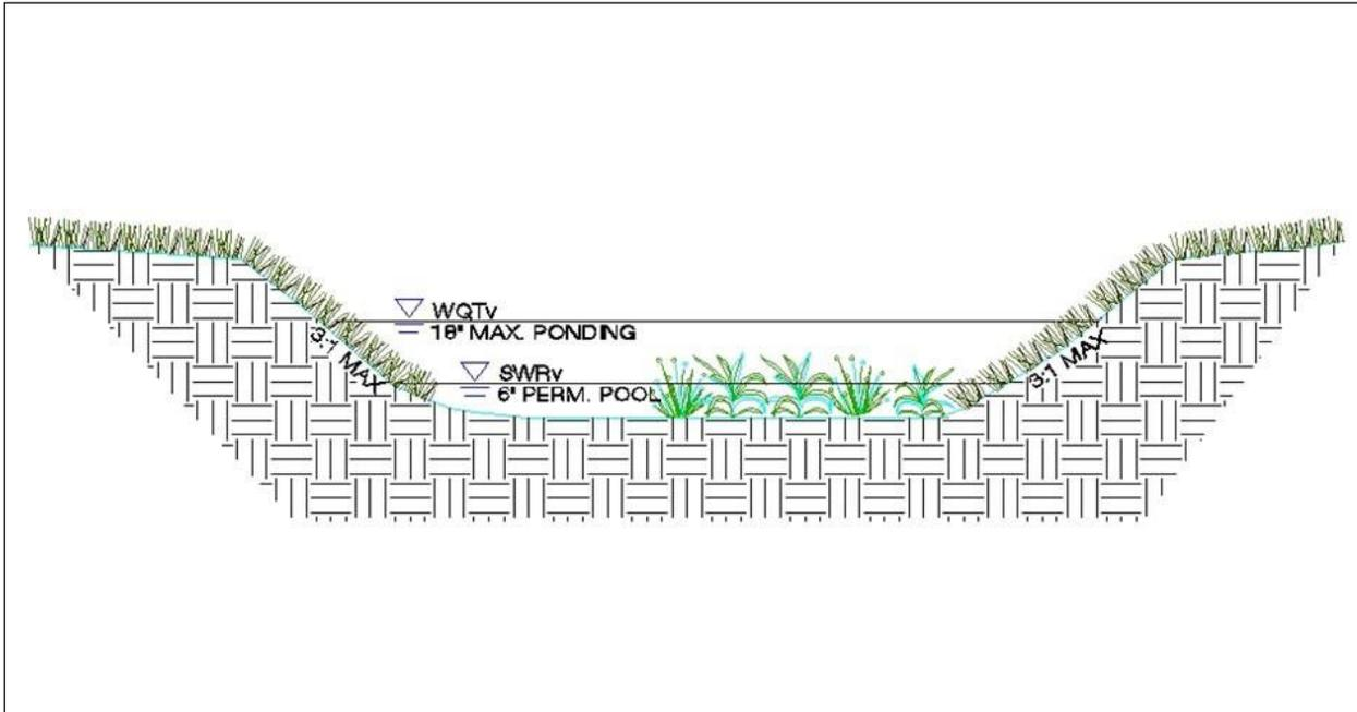
**Figure 4.36. Example of a wet swale (O-3).**
