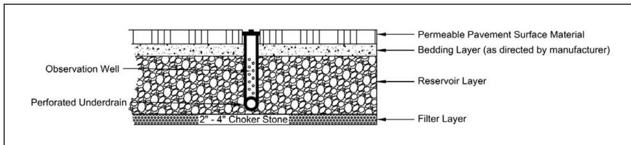
Figure 4.12. Cross-section of a standard permeable pavement design.
