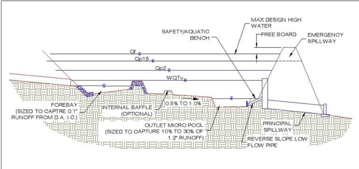
Figure 4. 51 Typical extended detention pond (C-3) details.
