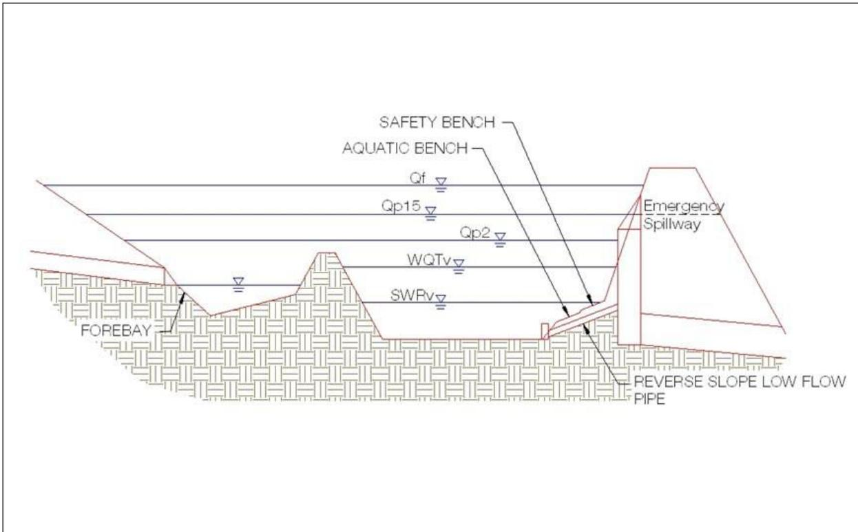
Figure 4. 50 Design schematics for a wet pond (C-2).
