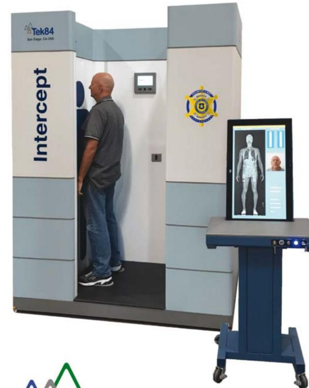
Detects both metallic and nonmetallic threats, including weapons, drugs, cell phones and other contraband. Screens from below the feet to above the head, revealing items under the clothing and within the body.
