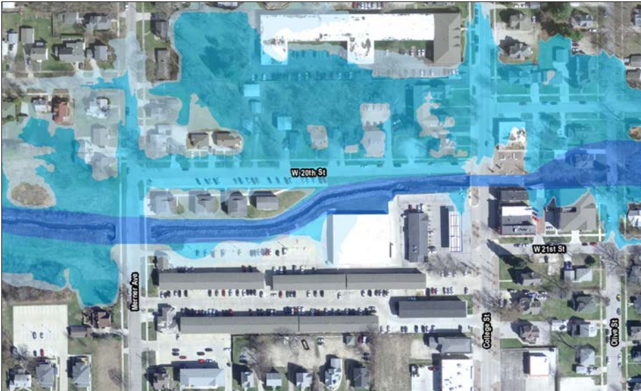
Dry Run Creek and the new reduced floodplain and floodway
