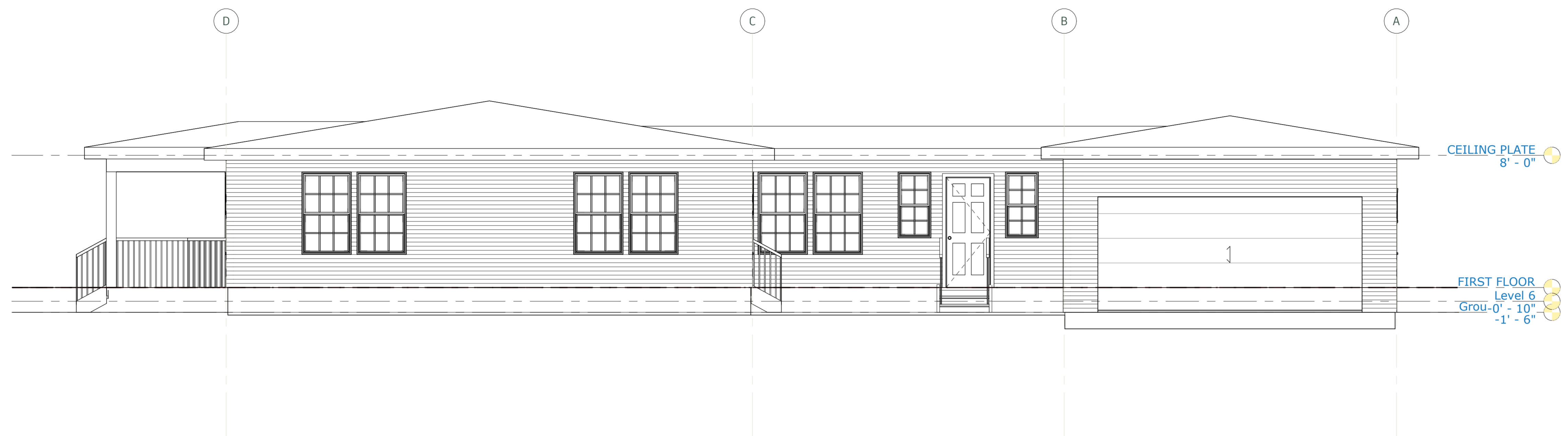
① EXISTING RIGHT ELEVATION 1/4" = 1'-0"
