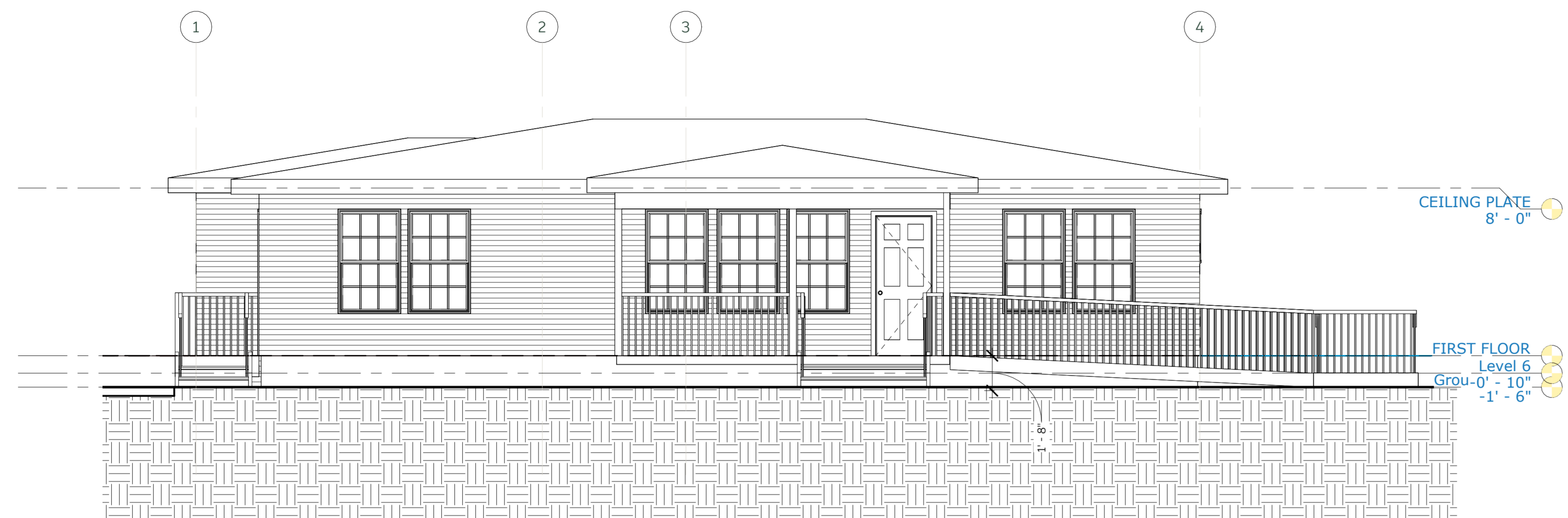
② NEW NORTH ELEVATION 1/4" = 1'-0"
