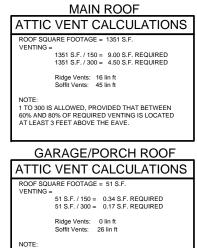
NOTE: 1 TO 300 IS ALLOWED, PROVIDED THAT BETWEEN 60% AND 80% OF REQUIRED VENTING IS LOCATED AT LEAST 3 FEET ABOVE THE EAVE.
