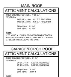
1 TO 300 IS ALLOWED, PROVIDED THAT BETWEEN 60% AND 80% OF REQUIRED VENTING IS LOCATED AT LEAST 3 FEET ABOVE THE EAVE.
