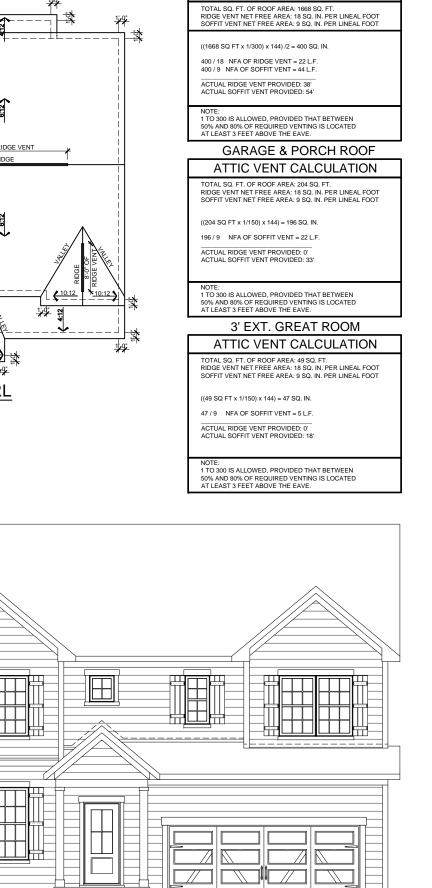
MAIN ROOF TRL ATTIC VENT CALCULATION
