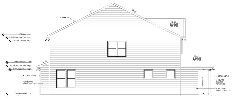
LEFT ELEVATION TRL SCALE: 1/8"=1"0" (11"x11" SHEET SIZE) SCALE: 1/4"=1"0" (24"x36" SHEET SIZE)
