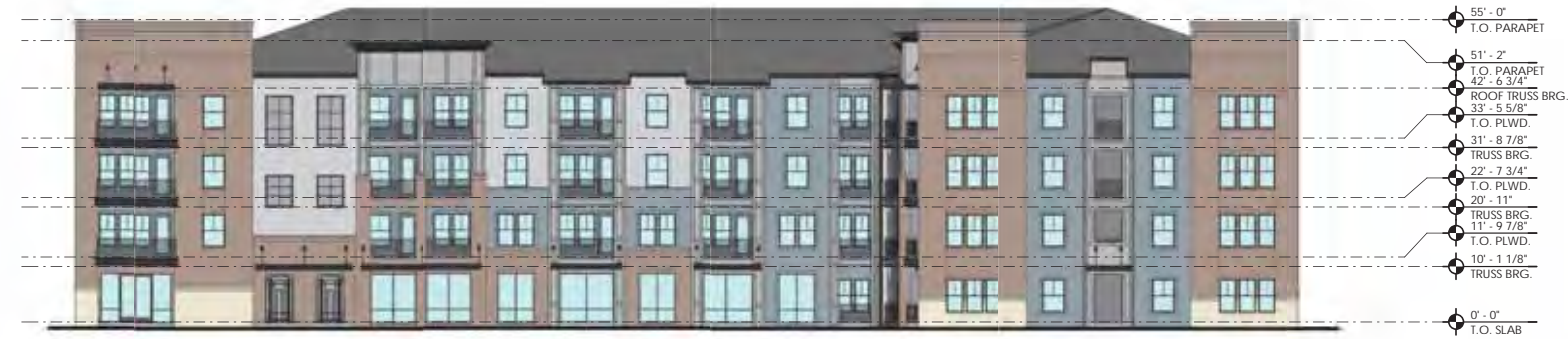
1 BUILDING TYPE I - OVERALL REAR ELEVATION SCALE: 1/16" = 1'-0"
