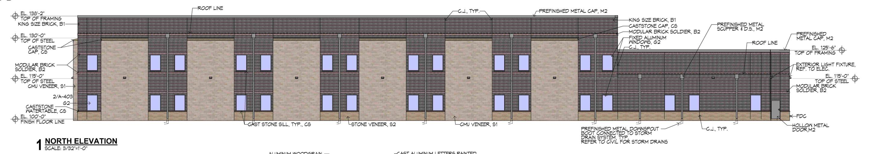
ALUMINUM MOODGRAIN -SIDING SYSTEM, M1 PREFINISHED METAL, COLOR TO MATCH M2 CAST ALUMINUM LETTERS PAINTED WHITE, 9" \$ 7" TALL LETTERS PREFINISHED — METAL CAP, M2 -ROOF LINE \_\_C.J., TYP.-EL. 138'-2"
