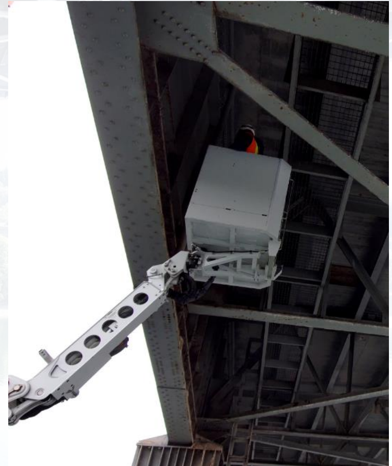
Inspection of inside girder during field test – note inspector cannot reach to upper part of girder
