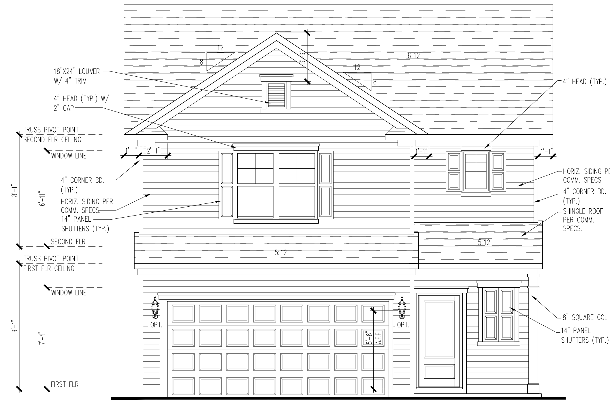
FRONT ELEVATION "LC1A" FRONT ENTRY GARAGE
