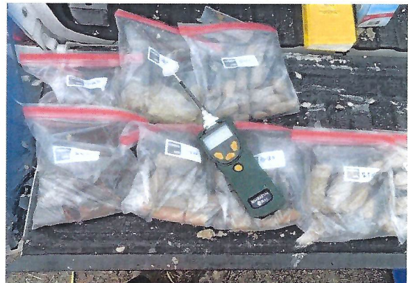
No. 4 View of soil recovered from SB-2 for soil screening, logging, and sampling.
