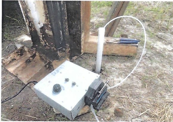
No. 7 View of temporary well at SB-3 for groundwater sample collection.
