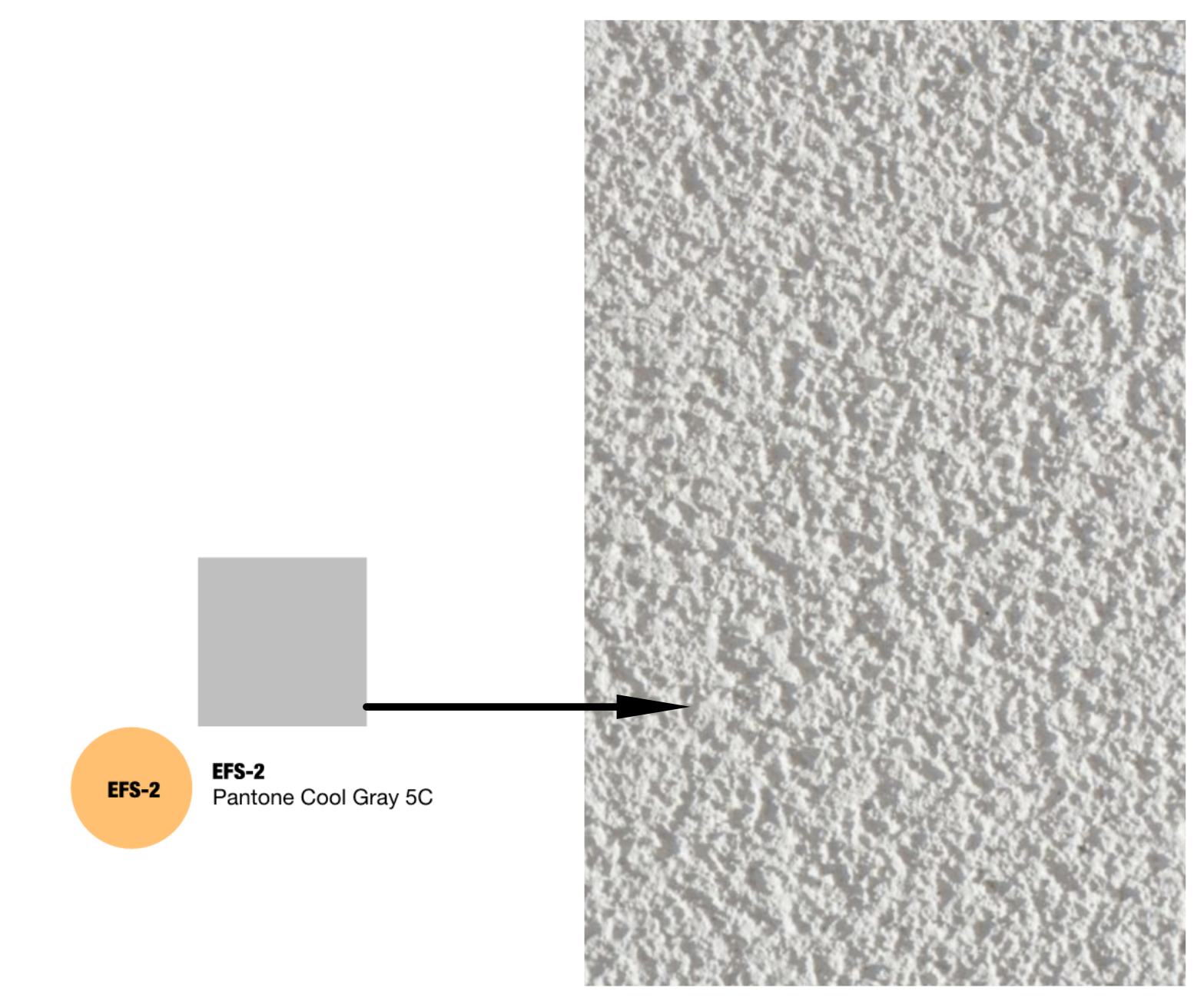
B Precast Concrete Upper body of building above 9'-0". Flat precast concrete panel with vertical pattern. Paint with medium texture EFS paint system in field.
