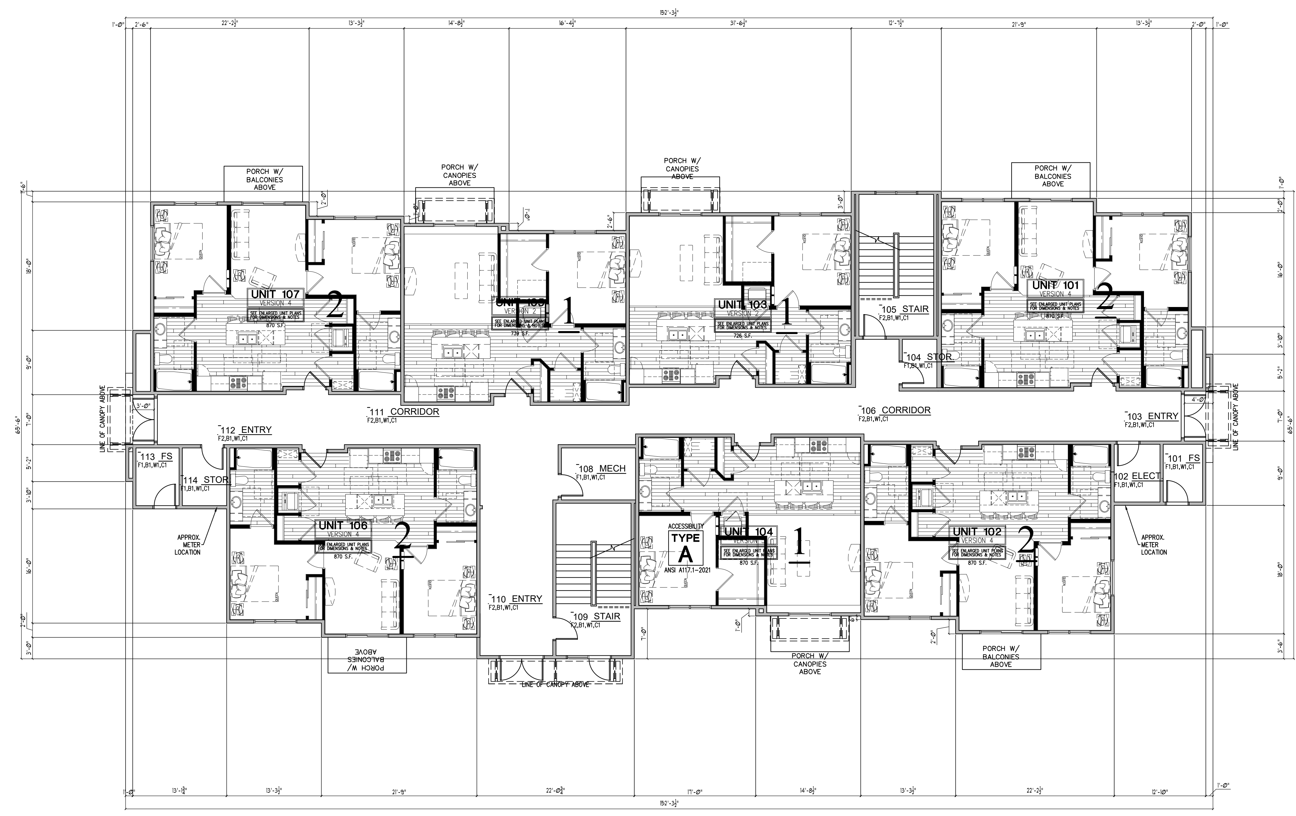
1 21 UNIT - LEVEL 1 - FLOOR PLAN (LEVEL 2 & 3 SIMILAR) SCALE: 1/8" = 1'-0" LEVEL 1 FLOOR PLAN ELEV. 100'-0" (DATUM) SEE CROSS SECTIONS SEE CIVIL DRAWINGS FOR EXTERIOR GRACES, CURBS, SIDEWALKS, AND OTHER SIMILAR SITE ELEMENTS APARTMENTS: (7 UNITS PER FLOOR) 5,815 SF ACCESSORY: 281 SF COMMON CORRIDOR & STAIRS: 2,022 SF TOTAL FLOOR AREA: 7,842 SF TOTAL APARTMENTS: (21 UNITS; 7 PER FLOOR) 17,445 SF TOTAL ACCESSORY: 783 SF TOTAL COMMON CORRIDOR & STAIRS: 6,081 SF BUILDING TOTAL FLOOR AREA: 24,309 SF
