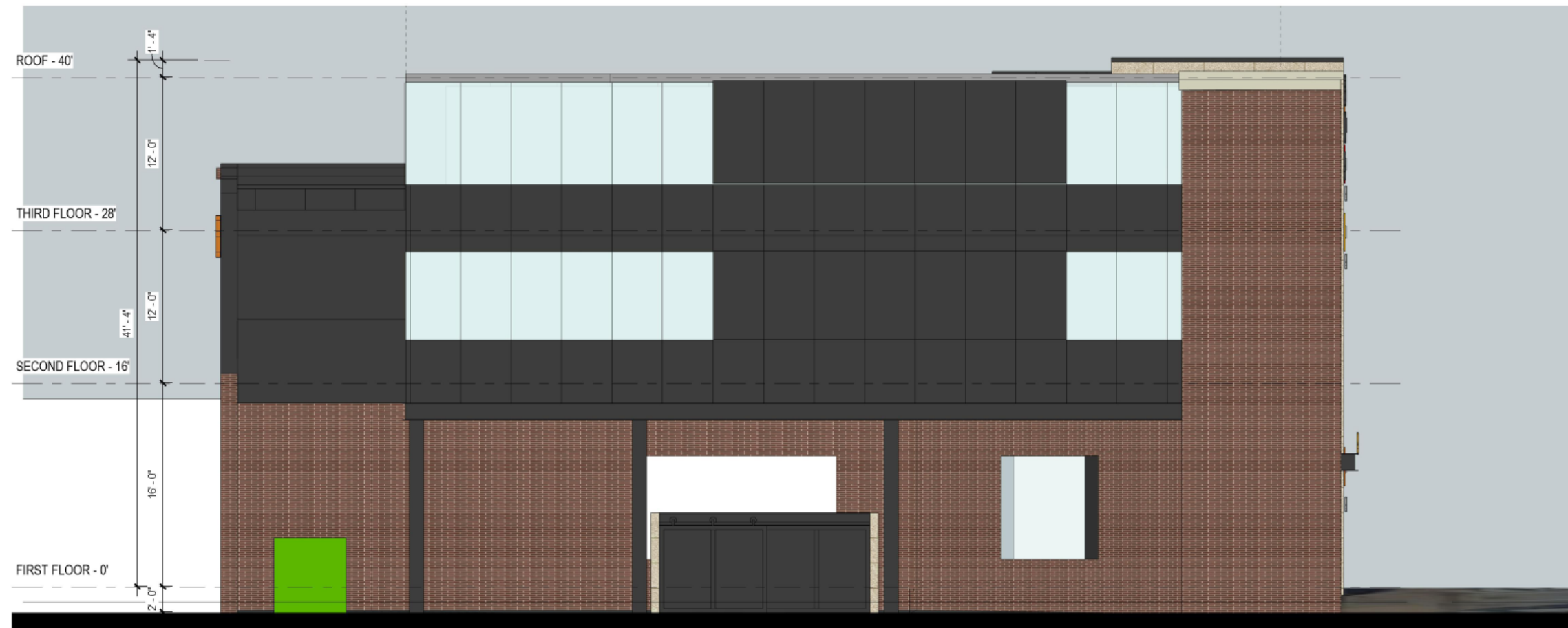
east elevation with heights
