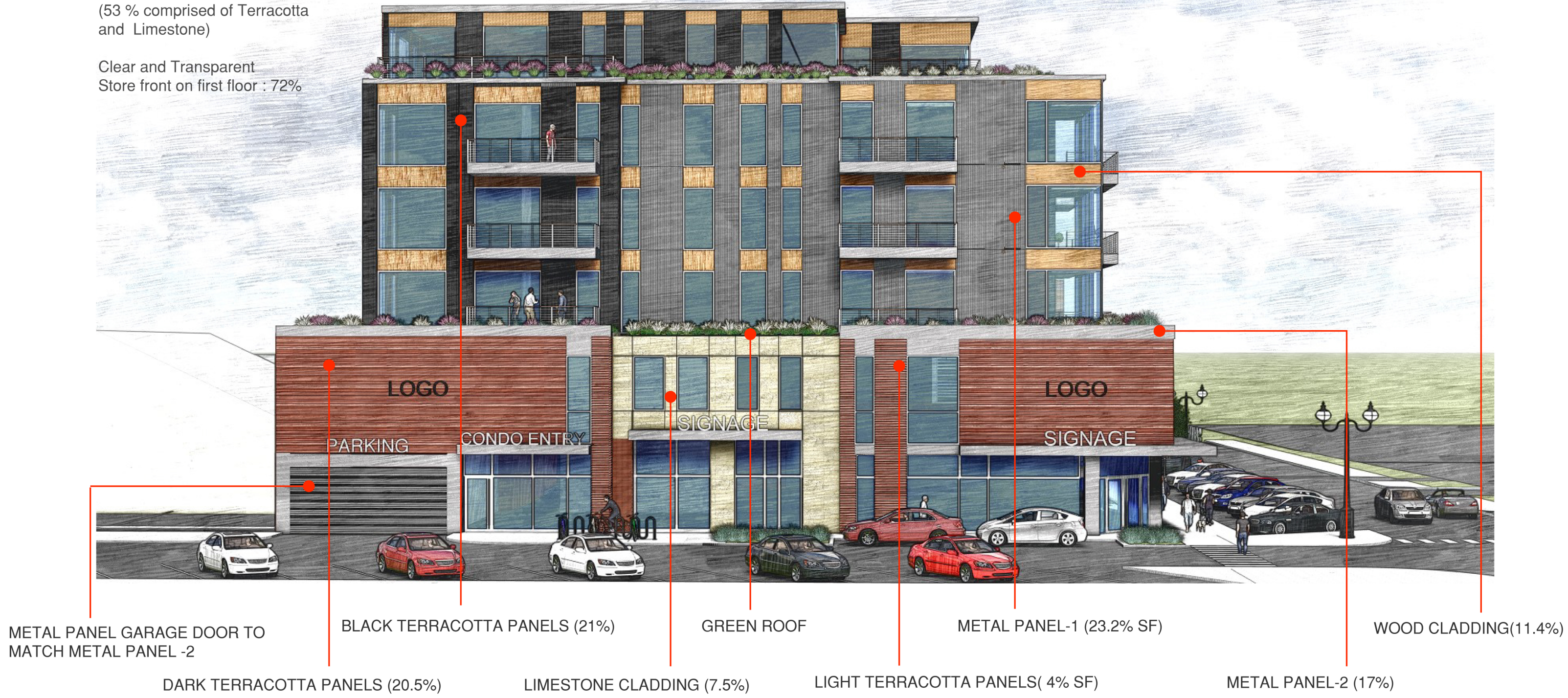
east elevation with material designations
