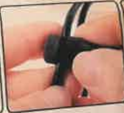
3. Twist the pin part into power cable tightly
