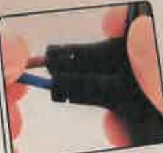
8. Pull test to make sure connect well
