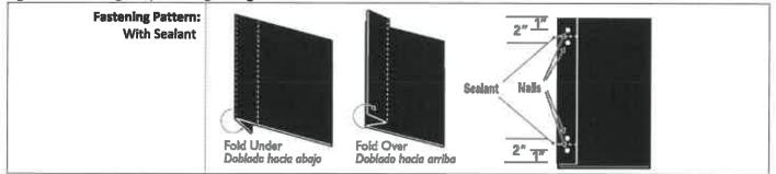
**DuraRidge™ Hip and Ridge Shingles:** Use two (2) fasteners per shingle. Fasten each shingle through the top laminated piece with one (1) fastener on each side, placed 9 inch from the exposed end and 1 inch in from the side edge. Fasteners must be located in the center of the SureNail<sup>®</sup> fastening area. See Figure 11 for fastener spacing. Maximum exposure to the weather must be 8 inches.
