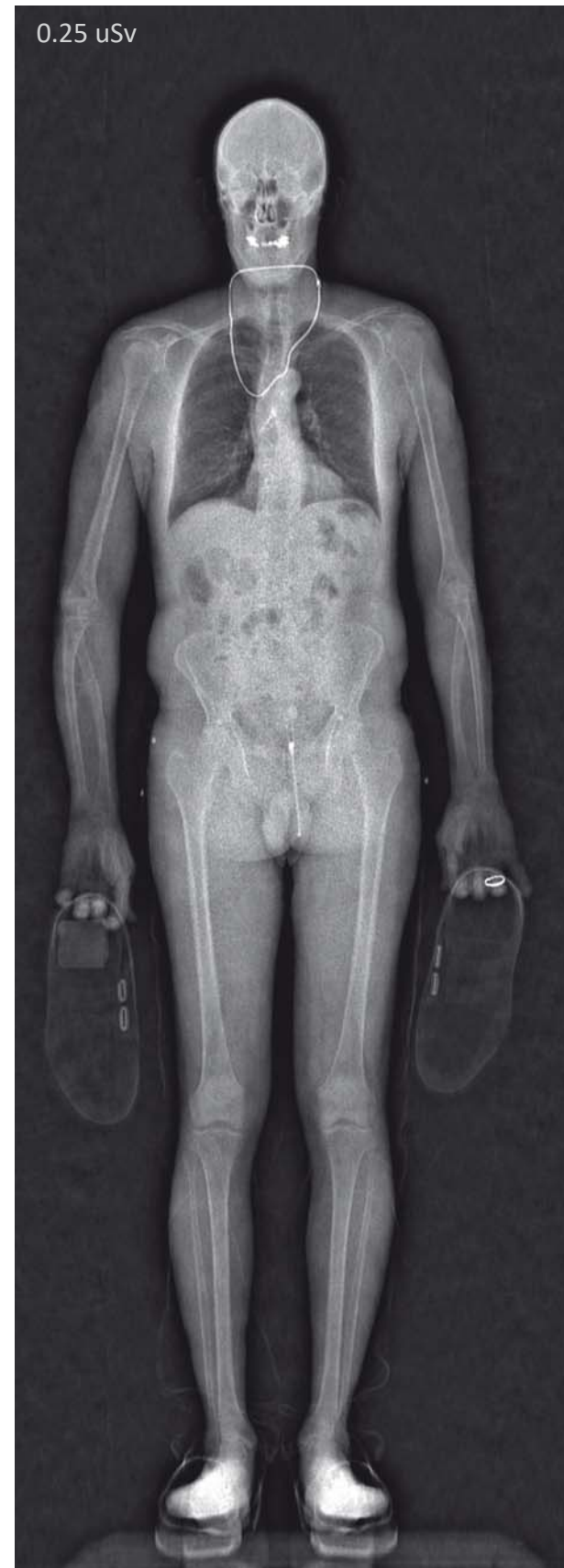
A typical image from Intercept on the lowest setting, 0.25 uSv. Items: teeth fillings, neck chain, object in shoe heel, ring and zipper. Intercept can operate at up to 200 uRem for even better image quality.
