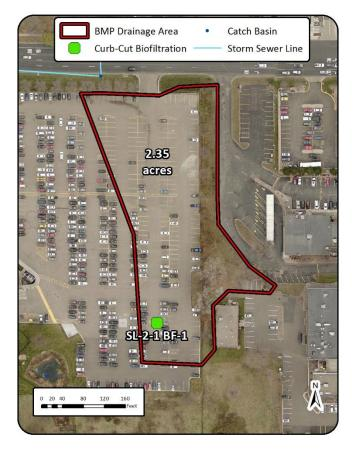
system. The potential site for this basin is adjacent to an existing catch basin, which could serve as the connection point for the underdrain outlet. The table below provides pollutant removals and estimated costs.
