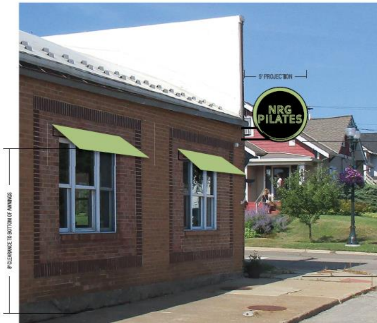
PMS 577 AWNINGS & PROJECTION SIGN TO BE INSTALLED WITH WEJ-IT ANCHORS AND EPOXY IF NEEDED
