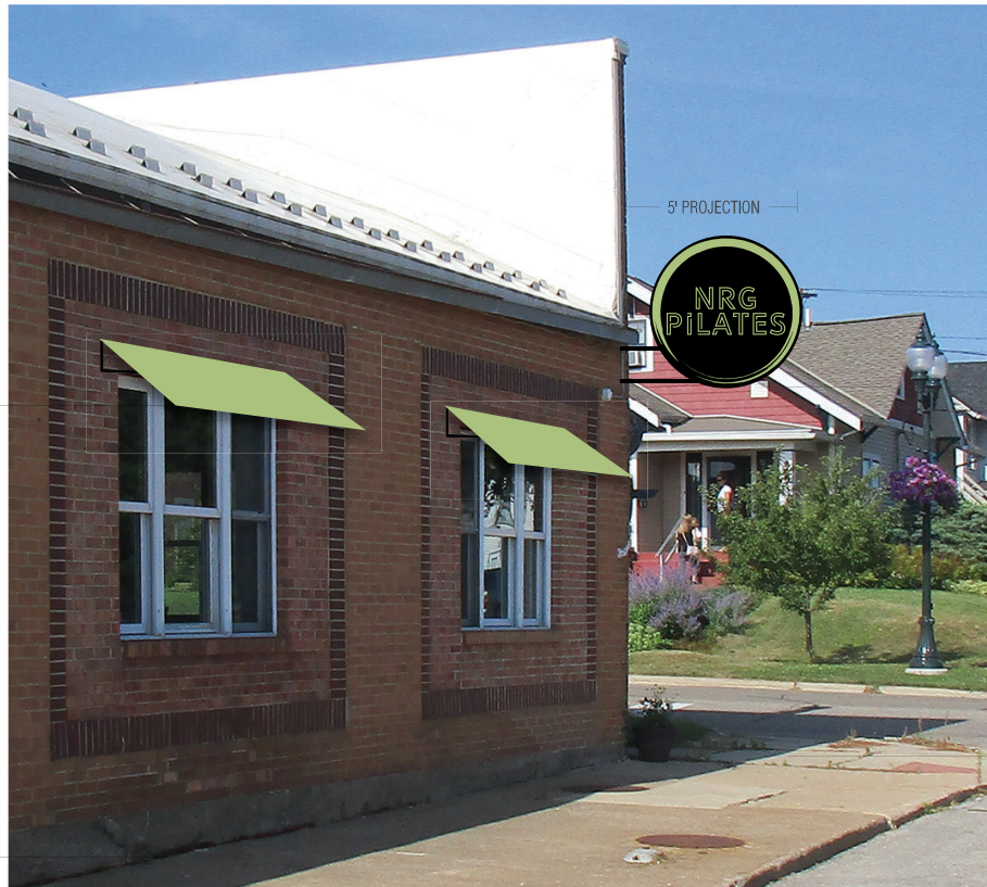
PMS 577 AWNINGS & PROJECTION SIGN TO BE INSTALLED WITH WEJ-IT ANCHORS AND EPOXY IF NEEDED
