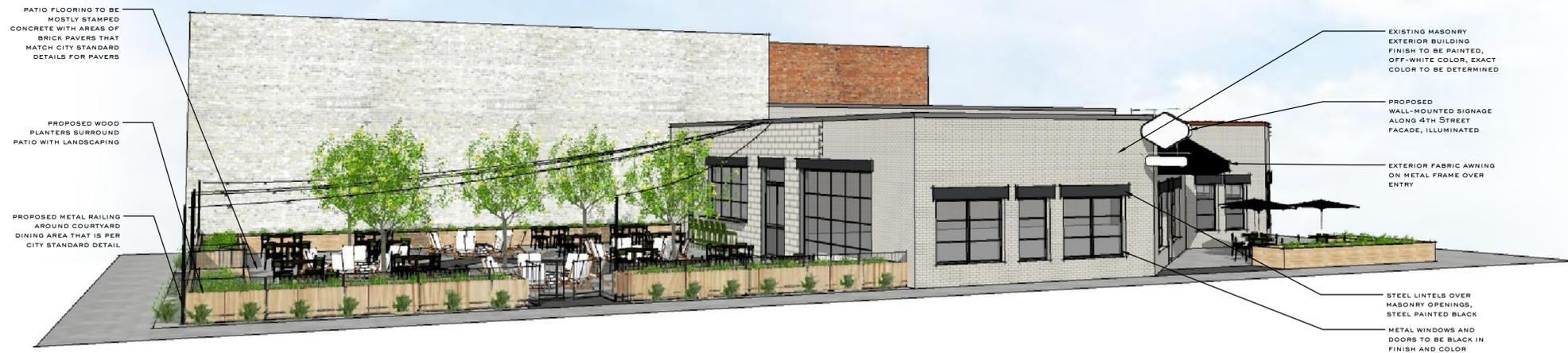
PATIO FLOORING TO BE MOSTLY STAMPED CONCRETE WITH AREAS OF BRICK PAVERS THAT MATCH CITY STANDARD DETAILS FOR PAVERS
