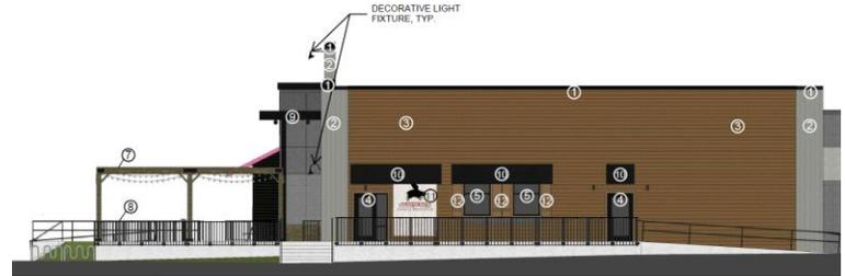
Proposed west elevation includes changing the façade to cedar lap siding in place of painted EIFS. Two vertical corrugated rustic metal panels will be added at both ends of the façade. Two doors are proposed one serving the entrance for customer and other leading to shared area of suites. The number of windows is reduced. Entire faced will be capped with firestone matt black color.
