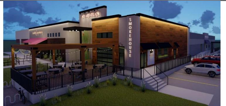
Proposed perspective view of the building shows the change of materials from EIFS to cedar lap siding (wooden), fewer awnings, increased header height along the north wall, increased height of canopy and wall sign and eliminating the projecting sign. Proposed work will also include a covering over the patio area.
