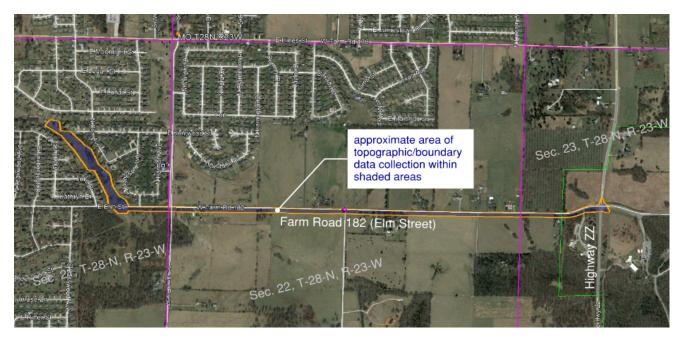
**Task 202:**Boundary Survey - The Consultant shall provide a list of horizontal control points with coordinates, descriptions, station and offset. Horizontal control will be based on the Missouri State Plane Coordinate System NAD 83–Central Zone-US Survey foot. Vertical control will be referenced to NAVD 88.
