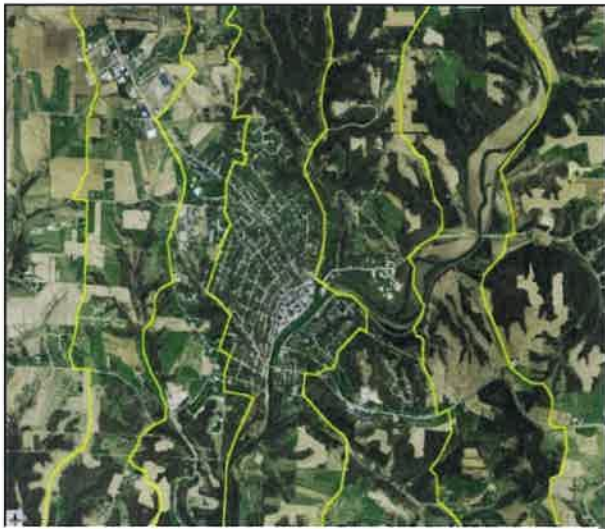
Figure 2: Mosaic after applying seams and balance. Instead of many "frames" in each flight strip there is only a single "strip" using the Leica ADS80 sensor. This simplifies and improves the quality of the mosaic due to less seams.
