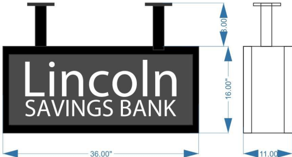
Signcomp standard extrusion.9" deep Acrylic faces Paint the frame and face to match the canopy.
