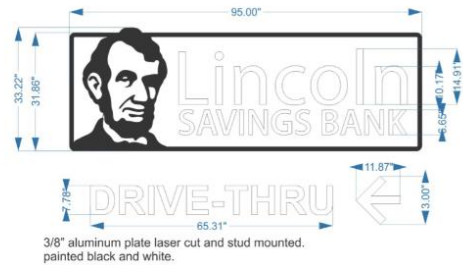
Non lighted Laser cut letters and logo Logo is 2' 10" x 8' ... 3/8" thick aluminum painted baked enamel. SIGNS & DESIGNS Drive Thru is 8" and arrow is 12" tall - same 3/8" thick aluminum.
