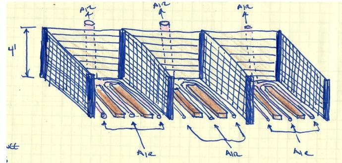
Railroad ties will be used as protective guides for the tractor bucket to slide on so that the piping isn't damaged.
