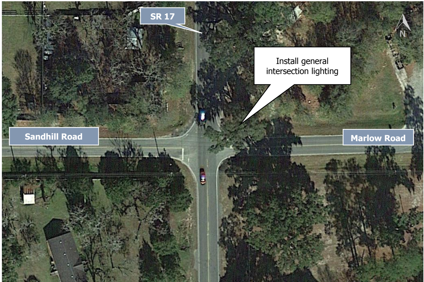
FIGURE 4-22. RECOMMENDED LIGHTING IMPROVEMENTS
