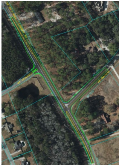
Figure 2-Left Turn Lanes-Secondary Alternative
