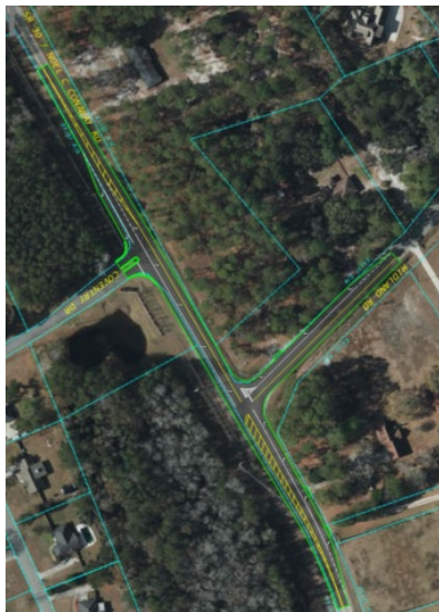
Figure 2-Left Turn Lanes-Secondary Alternative
