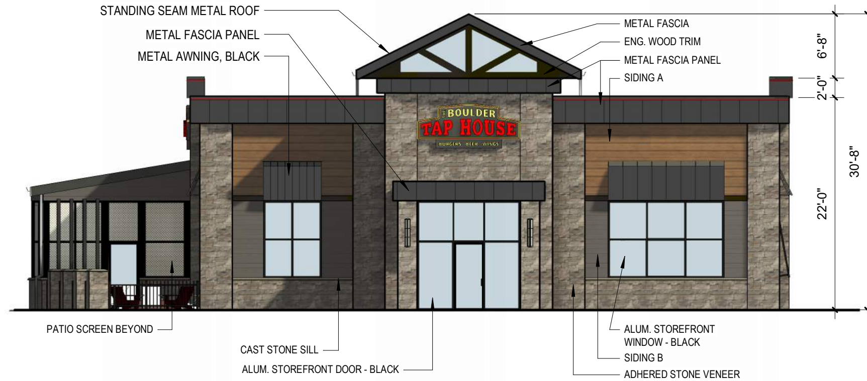
1 PROPOSED EAST ELEVATION 1" = 10'-0" FENESTRATIONS = 25%
