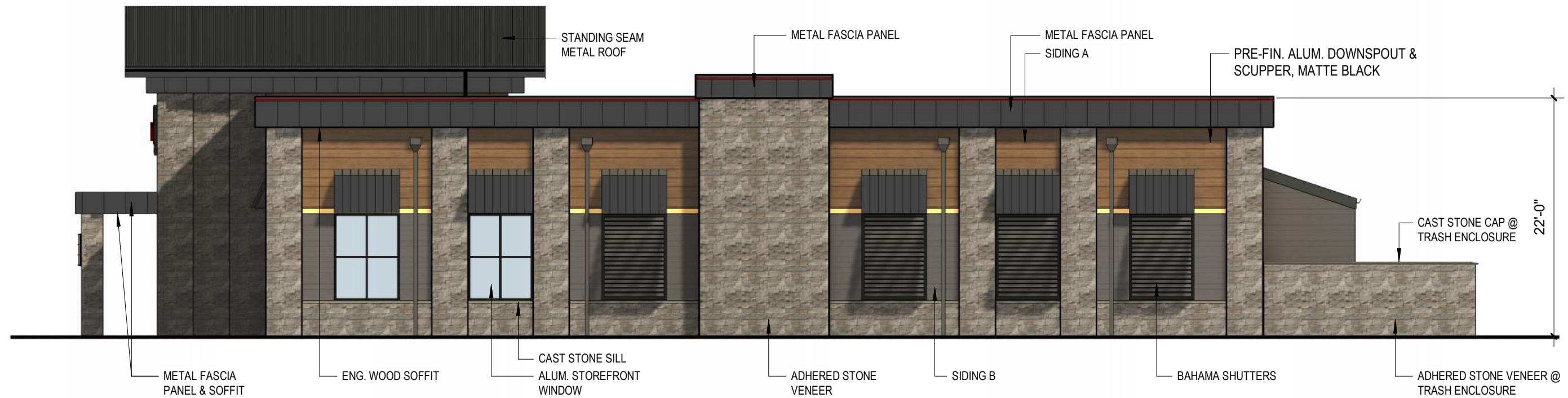
2 PROPOSED NORTH ELEVATION 1" = 10'-0" FENESTRATIONS = 14%
