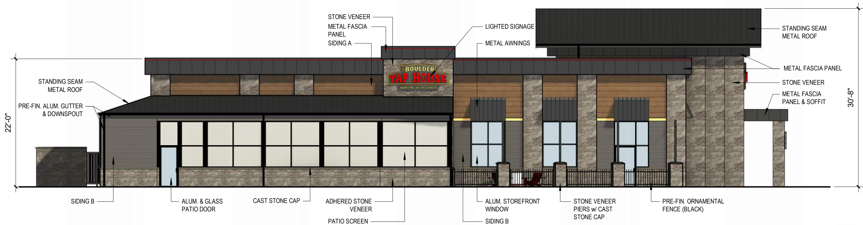
1 PROPOSED SOUTH ELEVATION 1" = 10'-0" FENESTRATIONS = 26%
