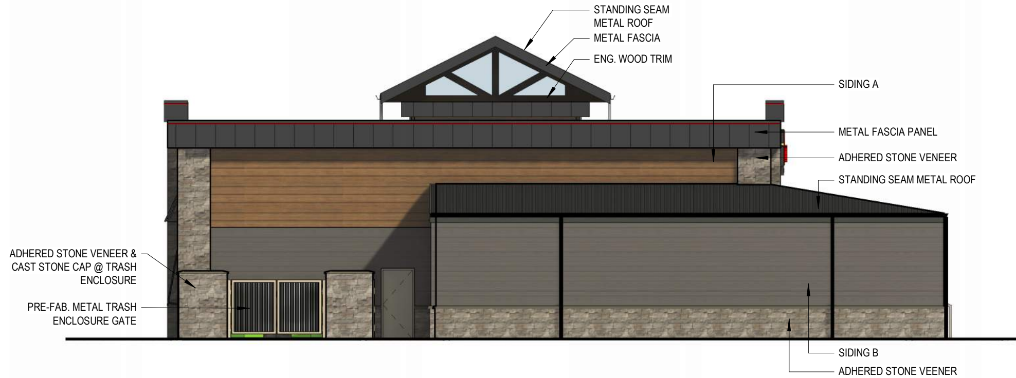
2 PROPOSED WEST ELEVATION 1" = 10'-0" FENESTRATIONS = 2%
