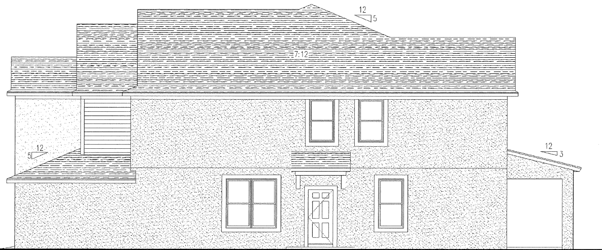
BUILDING TYPE 8B - RIGHT ELEVATION SCALE: 3/16"=1'-0"
